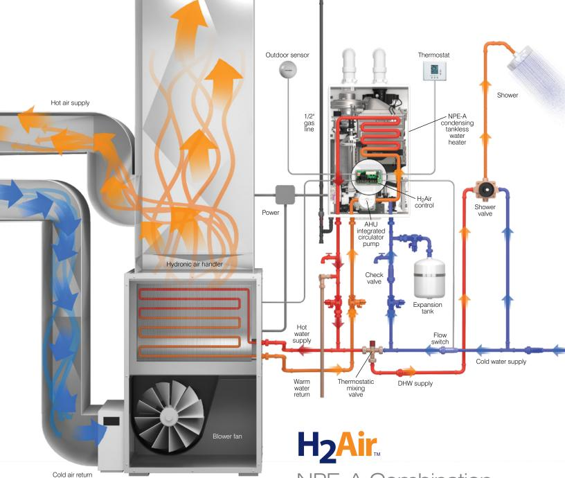
H<sub>2</sub>Air is compatible with hydronic air handler models that require W1/W2/R terminals along with single or dual-stage thermostats.\*\*
